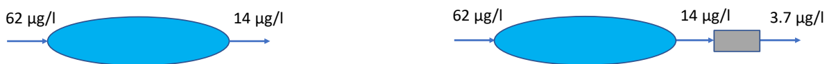
Figure 1. To the left a wet pond treating the stormwater and to the right a wet pond combined with a smaller underground retention filter basin.
