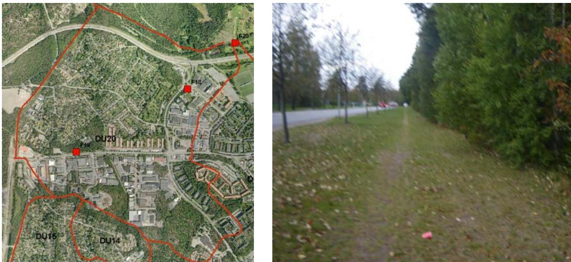
**Figure 4** To the left proposed detention measures for reducing floods in one of the subwatershed areas in Lindalen, Tyresö. To the right the proposed place for a dry detention pond, adjacent to the road Bollmoravägen in Tyresö.
